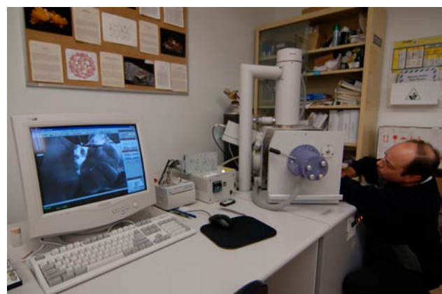
Figure 3. Mr. Paul Hamilton places a specimen in the vacuum chamber of the environmental scanning electron microscope.
