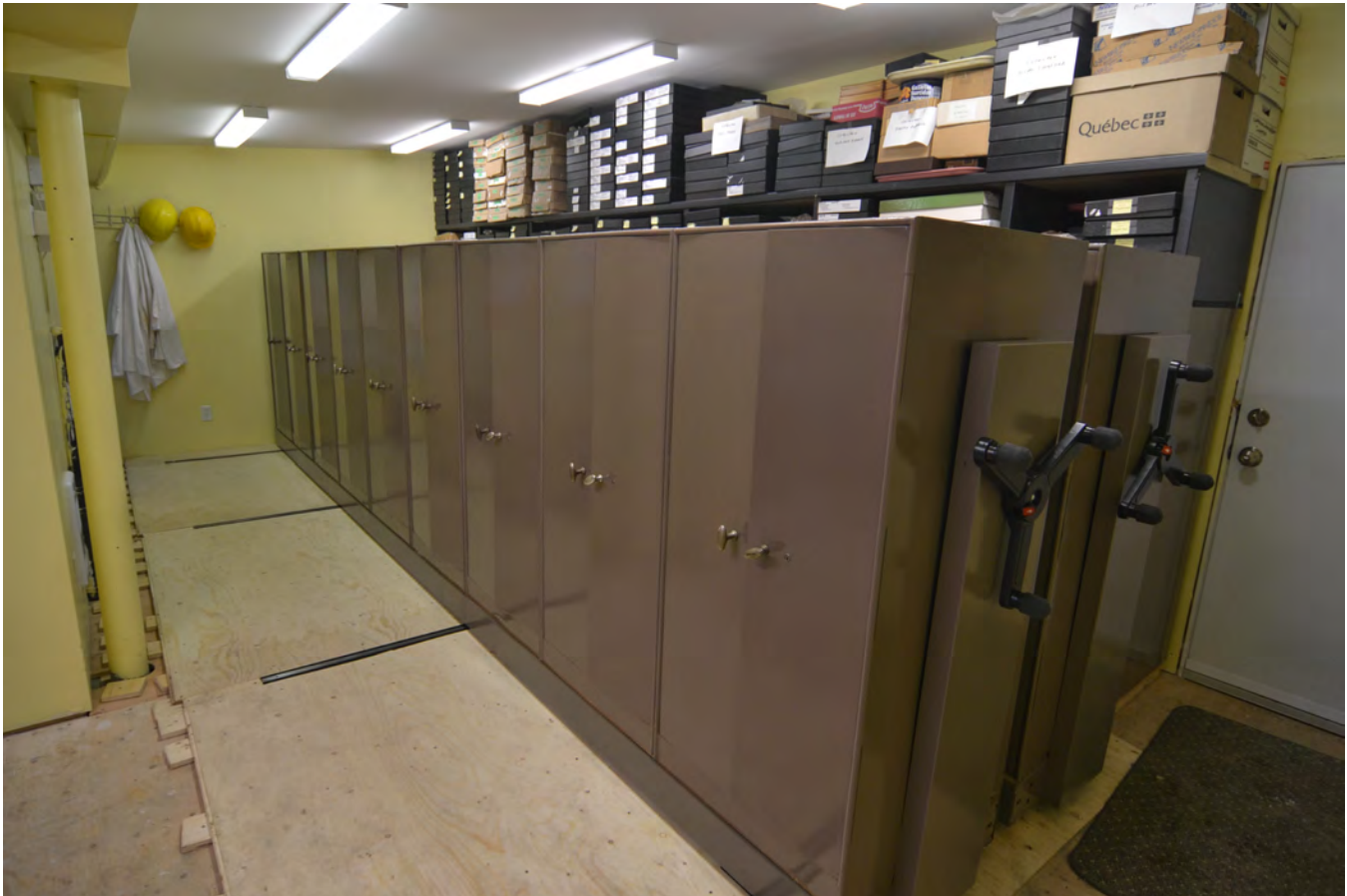
The new room at the Laboratory for Conservation and Research - MPE with its new high-density mobile storage system. The mobile trolleys were custom made to accommodate our "Bankers Cabinets," which had been given to us by the Canadian Museum of Nature, a few years ago.
